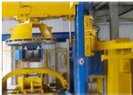
Schlüssellbauer vertical cast equipment capable of making Pipes, Box Culverts & Manholes.
