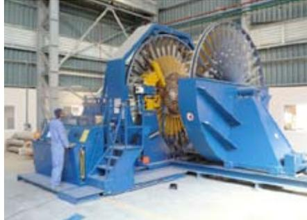
MBK Cage Welding Machine can make cages in diameters ranging from 300 millimeters to 3600 millimeters.
